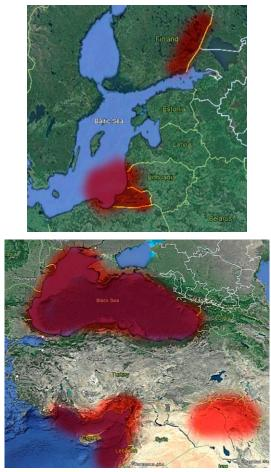
Images based on description provided in EASA, "Safety Information Bulletin - Global Navigation Satellite System Outage Leading to Navigation / Surveillance Degradation,". 2022
